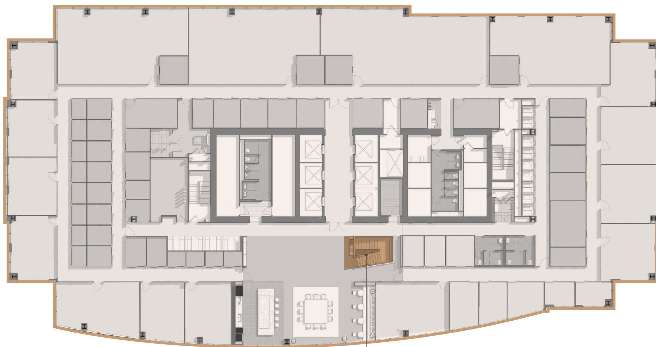
INTERNAL STAIRCASE CONNECTING TO FLOOR 20
